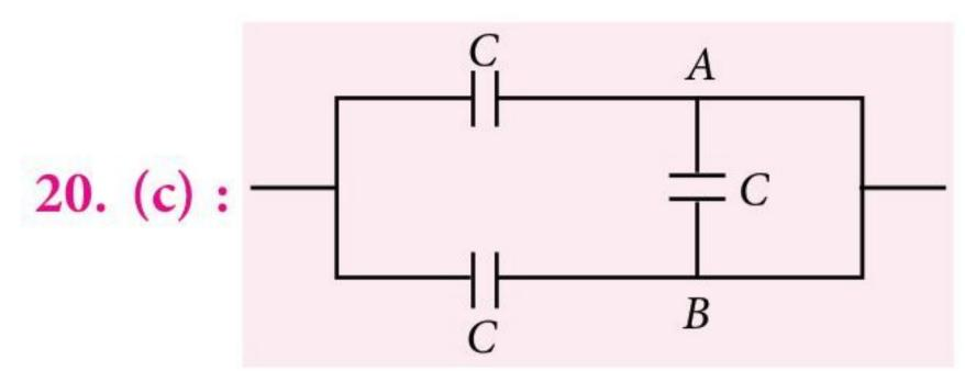
Here, AB arm is short, so the two capacitors C and C in parallel,  $C_{eq} = C + C = 2C$
