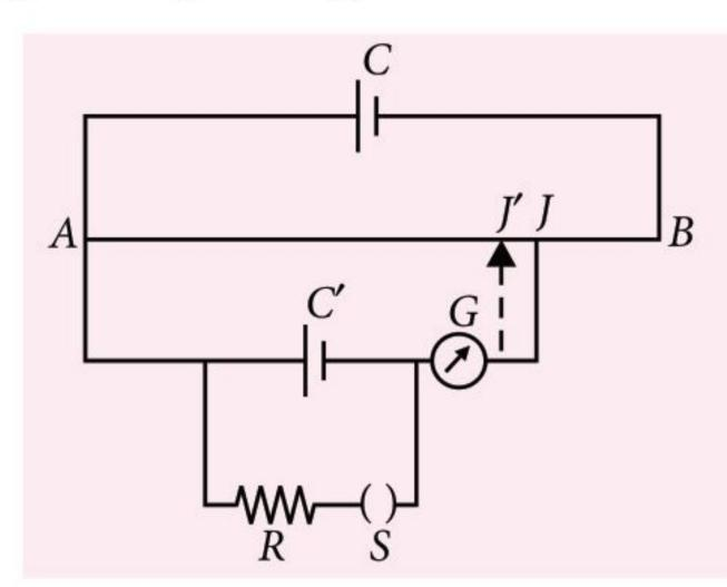
Let  $\varepsilon$  be the emf of the cell C' and r its internal resistance. Let l = AJ be the balance length when switch S is open. When a resistance R is introduced by closing the switch a current begins of flow through the cell C' and resistance R. The potential difference between the terminals of the cells falls and the balance length decreases to l' = AJ'. The terminal resistance of the cell is given by
