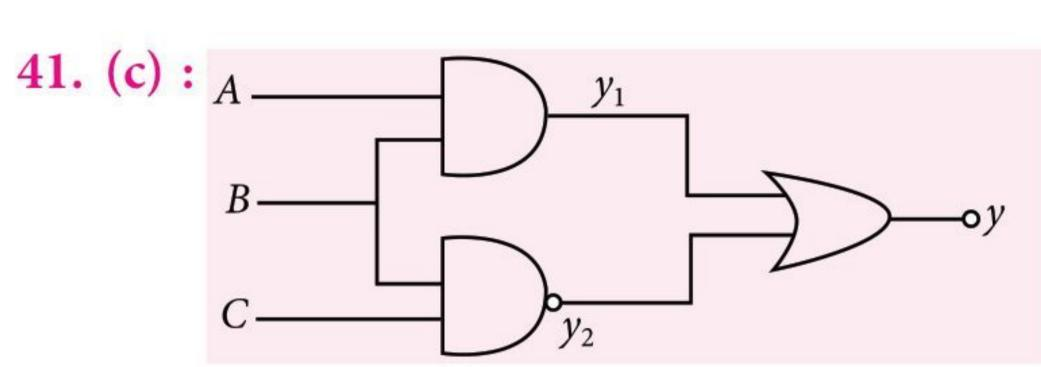
Output of combination of logic gates is given as
