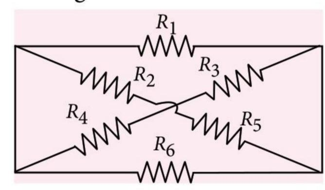
$R_1$ ,  $R_S'$ ,  $R_S''$  and  $R_6$  are in parallel.
